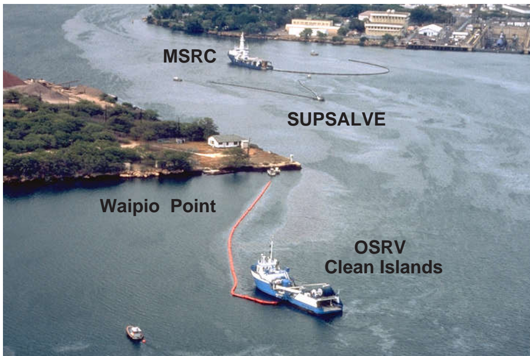
The OSRV Clean Islands works with MSRC and SUPSALVE to collect free floating oil.
